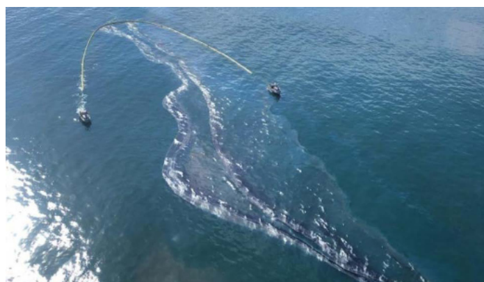
Crude oil in the Pacific Ocean off the California coast on October 3, 2021. Oil spill removal organization vessels are towing a skirted oil boom to contain the oil spill.
