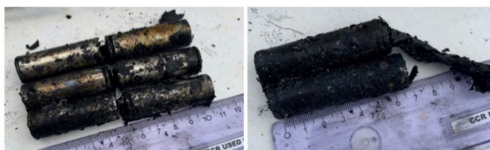
Figure 8. The nickel-metal hydride battery's cells (left) and remains of the lithium-ion battery cells and components (right) found on the communications table. (Source: ATF)
