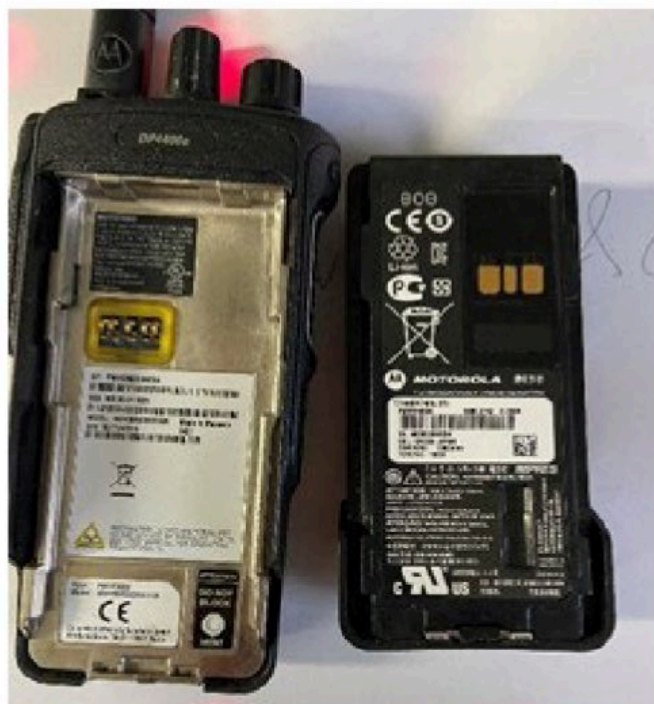
Figure 6. A Motorola DP4400e radio and lithium-ion battery used on the bridge of the S-Trust .
